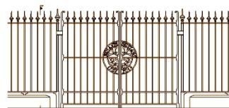
Figure 23 Proposed north gate to Inverleith Place. S&B
